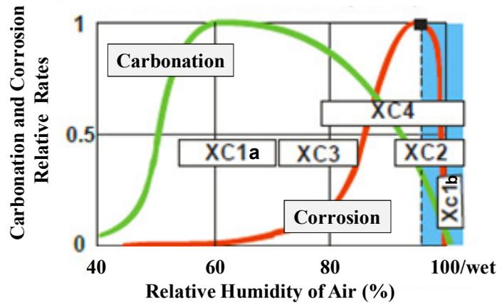
Fig. 2 - Carbonation and corrosion relative rates as function of RH of air [22]
