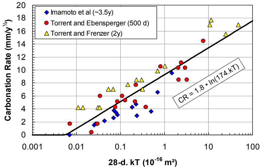
Fig. 1 - Correlation between Carbonation Rate and Coefficient of Air-Permeability kT [14-16]
